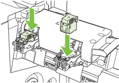
7. Pull the handle of the staple cartridge unit toward you and rotate it downward to its original position. Lock it into position by pushing in the handle.
