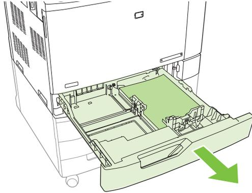
6. Pull the tray completely out of the product by pulling and lifting it up slightly.
