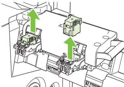
5. Unpack the new cartridges and remove the plastic packing lock from each one.
