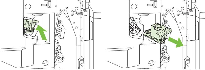
3. Insert the replacement staple cartridge unit into the stapler unit.
