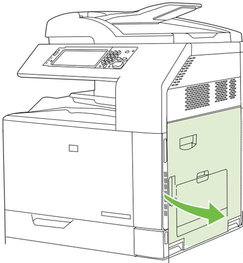
2. If paper is visible inside the right door, gently pull the paper downward to remove it.
