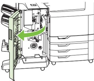
2. Push the upper delivery guide to the right, and remove any jammed paper.
