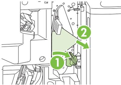
5. The positioning knob is the smaller, green dial on the right. Turn the positioning knob counterclockwise.
