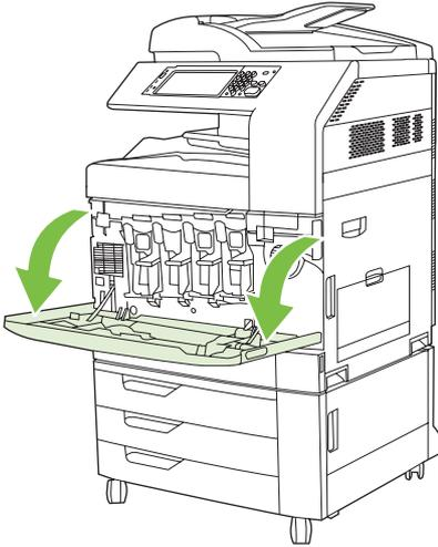
2. Grasp the handle of the used print cartridge and pull out to remove.
