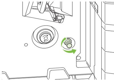
6. The jam-release knob is the larger, green dial on the left. Push in the jam-release knob, and then turn it clockwise to move any jammed paper into the output bin.
