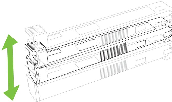
7. Align the print cartridge with its slot and insert the print cartridge until it clicks into place.
