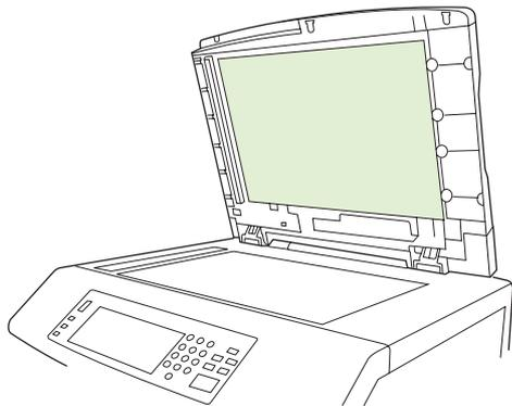
3. Clean the ADF backing by wiping them with a clean, damp, lint-free cloth. Use an ammonia-based surface cleaner only when a water-dampened cloth does not clean the ADF components.
