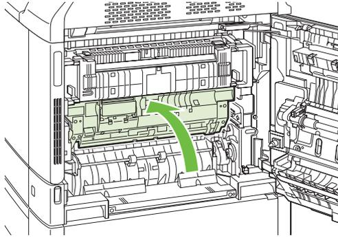
5. Open the fuser jam access door above the fuser and remove any paper that is visible. Then close the fuser jam access door.
