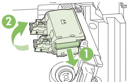
4. Grasp the edges of each staple cartridge and pull up firmly to remove the staple cartridges from the staple cartridge unit.
