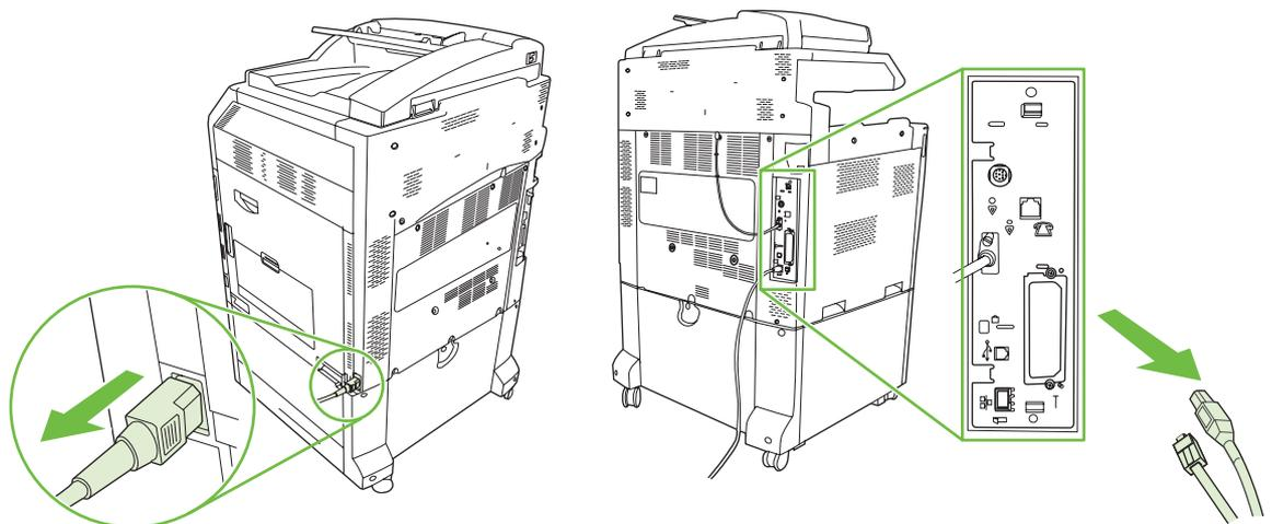
3. Locate the black formatter pressure release tabs on the formatter board in the rear of the product.
