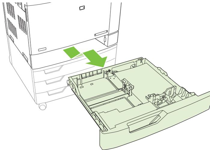
7. Remove any paper from the feeder rollers inside the product.
