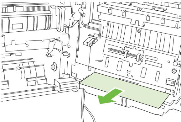
3. If paper has entered the internal paper path, lift the green handle on the transfer-access panel and open the panel.
