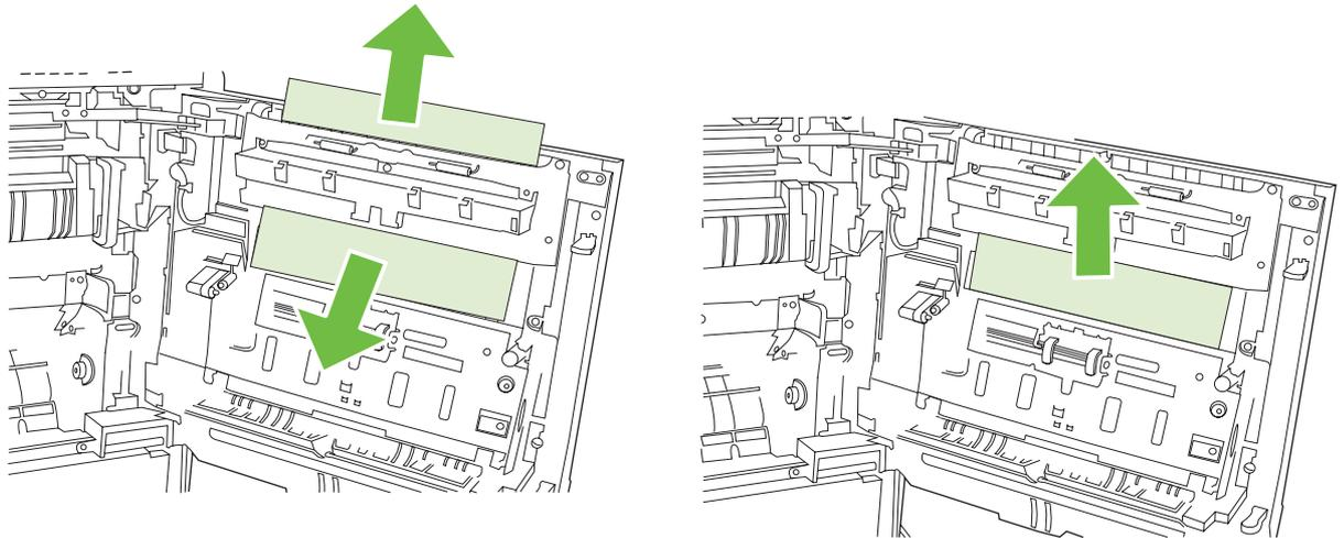
4. Lift the paper-feed cover on the inside of the right door. If jammed paper is present, gently pull the paper straight out to remove it.
