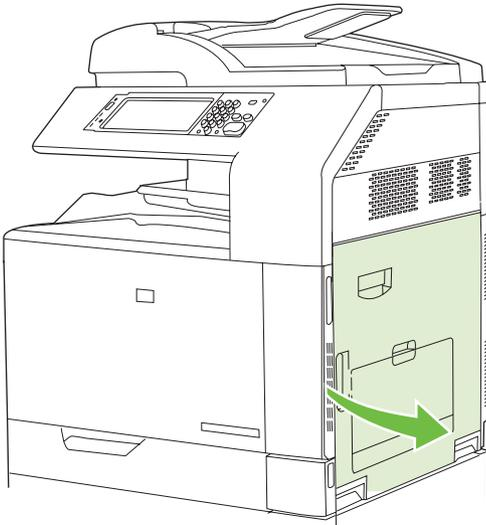
2. If paper is jammed below the duplexing unit, gently pull the paper downward to remove it.
