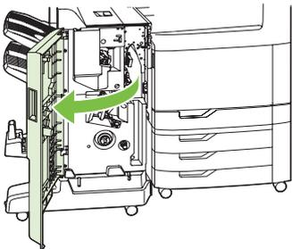
3. Push the upper delivery guide to the right, and remove any jammed paper.
