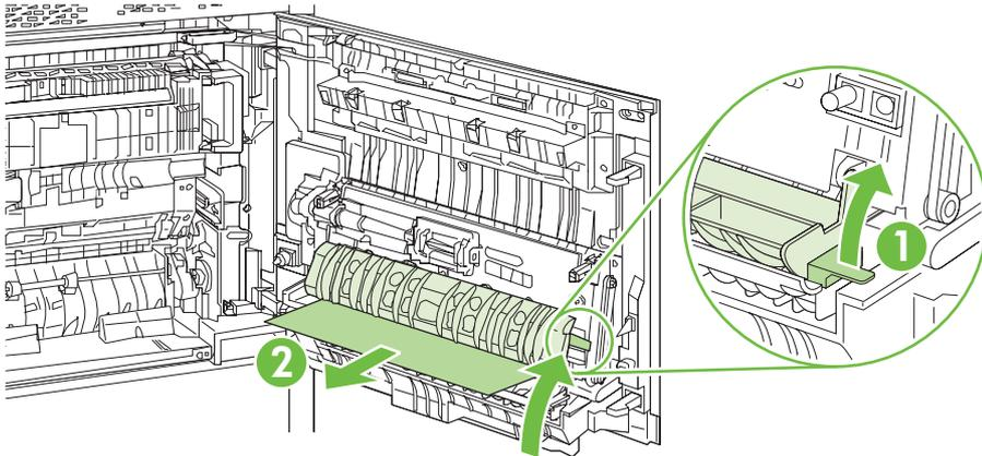
5. Lift the green handle on the transfer-assembly and open the panel.
