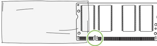
8. Holding the DIMM by the edges, align the notch on the DIMM with the bar in the DIMM slot at an angle and firmly press the DIMM into the slot until it is fully seated. When installed correctly, the metal contacts are not visible.
