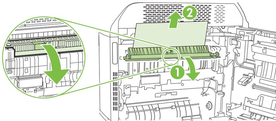
6. Paper could also be jammed inside the fuser where it would not be visible. Remove the fuser to check for jammed paper inside.
