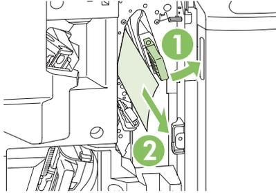
3. Grasp the blue handle for the stapler carriage and pull it straight out.
