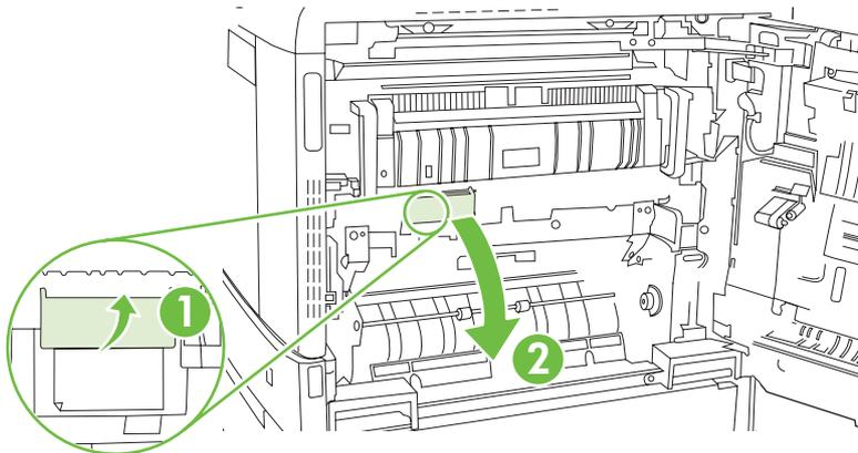
3. If paper is visible entering the bottom of the fuser, gently pull downward to remove it.
