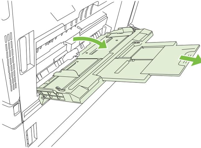
2. Set the side guides to the correct width, and pull out the tray extensions to support paper.
