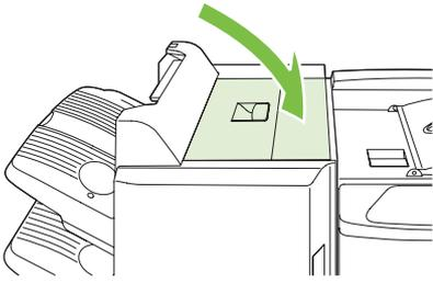
4. Lift the swing guide panel in the output bin. If you can see any jammed paper, gently pull it out.
