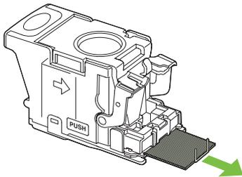
5. Close the lever at the back of the staple cartridge. Be sure that it snaps into place.
