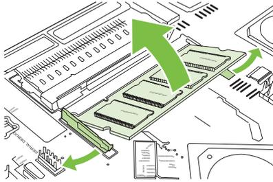
7. Remove the new DIMM from the antistatic package. Locate the alignment notch on the bottom edge of the DIMM.
