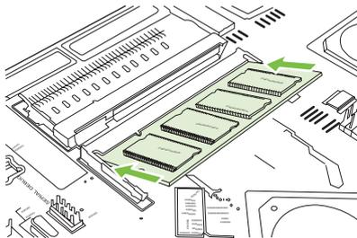
9. Push down on the DIMM until both latches engage the DIMM.
