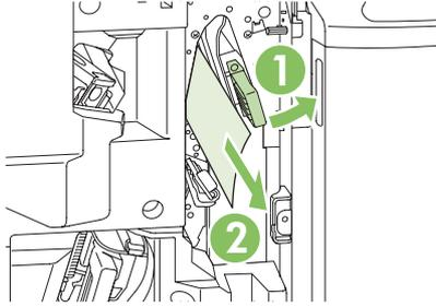
4. Push the lower delivery guide to the right, and remove any jammed paper.
