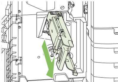
4. Grasp the handle of the blue staple cartridge unit and pull it toward you, then swing the staple cartridge unit into an upright position.
