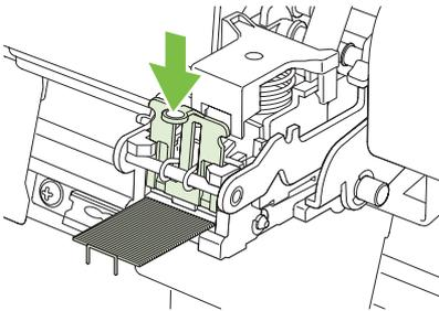
6. Pull the staple cartridge unit forward, and swing it downward to the original position. Push in on the handle to lock it into position.
