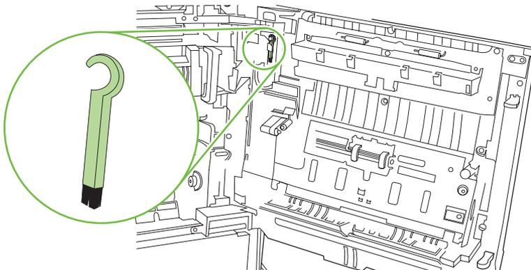
3. Lift the green handle on the transfer-access panel and open the panel.
