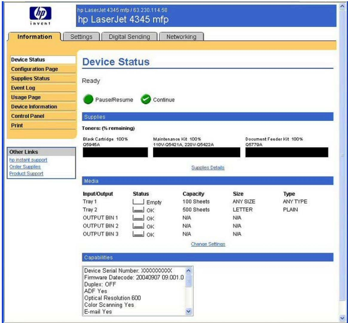
Figure 2-1 Device Status screen on the Information tab
