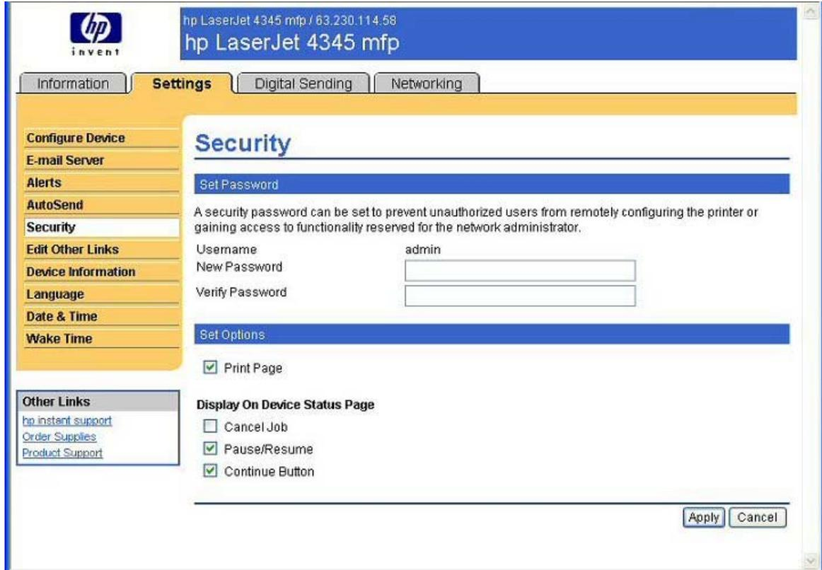
**Figure 2-5** Security screen on the **Settings** tab
